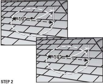
Hammer a nail at the center of the location chosen between rafters for the Greenergy Solar Attic Fan. The center of the unit should be about 2 feet down from the ridge.
