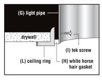
snips. Secure bottom of light pipe to ceiling ring with two tek screws (I). NOTE: Use caution, light pipe is extremely sharp.
