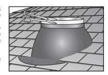
is extremely sharp. STEP 17 Place dome (A) on top of the flashing unit (E). Secure the dome to the flashing
