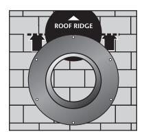
STEP 11 Apply caulk over all exposed screw heads (since they will be exposed to the weather). Use remaining caulk to seal the areas where the 4" slits were made and around area where shingles meet with raised area of the flashing.
